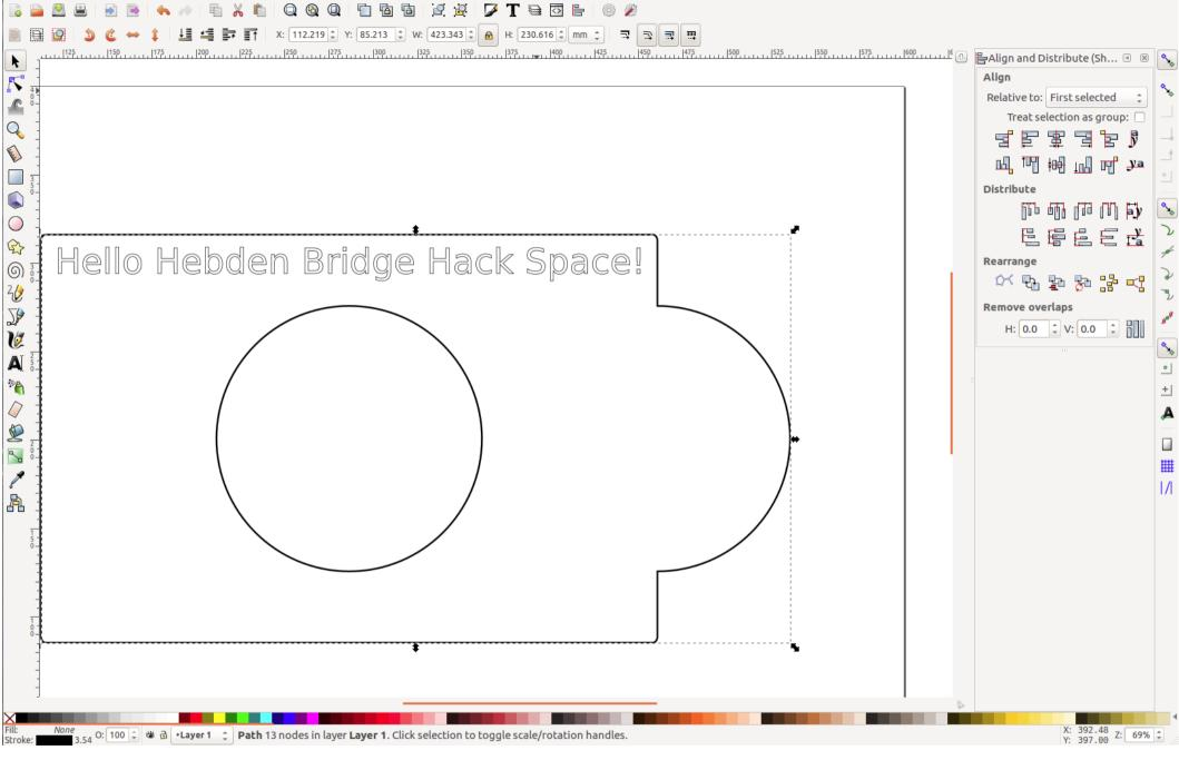
This is the union of the original shapes. Select both using Shft+Ctrl+\*select  $1^{st}$  object\*+\*select  $2^{nd}$  object\* then Path > Union
