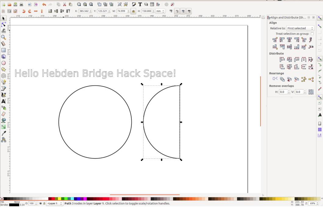
This is the intersection of the original shapes. Select both using Shft+Ctrl+\*select  $1^{st}$  object\*+\*select  $2^{nd}$  object\* then Path > Intersection
