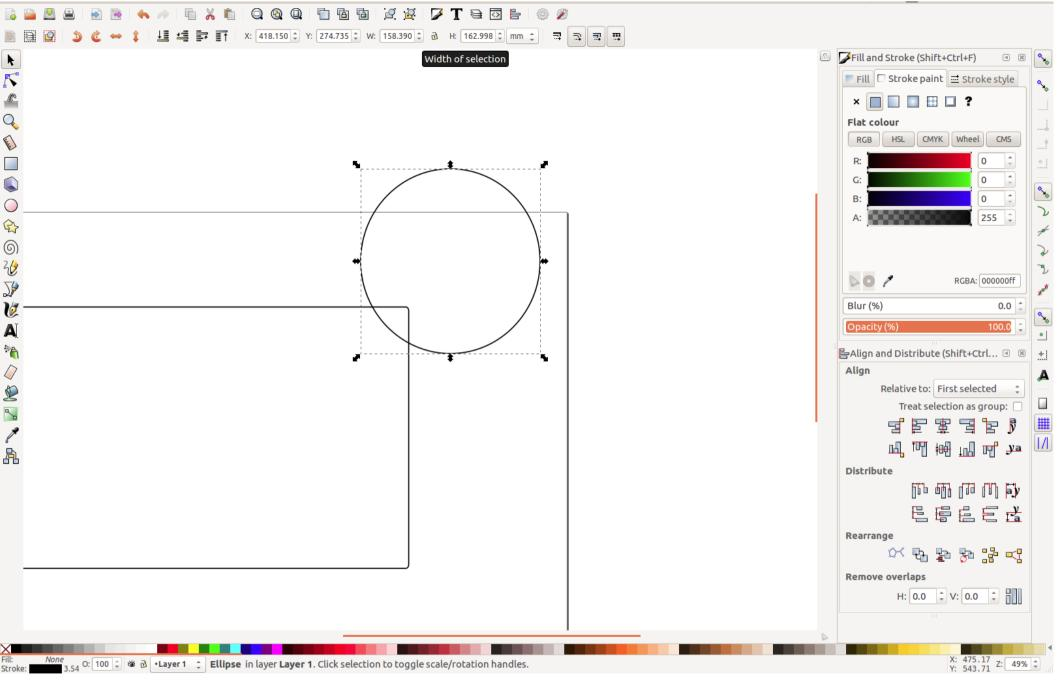
When we draw a circle using the toolbar it isn't perfectly round. To change the properties of this we make the width and height the same (top toolbar when circle is selected). If we 'lock' this it keeps the scale even though the diameter can be changed.
