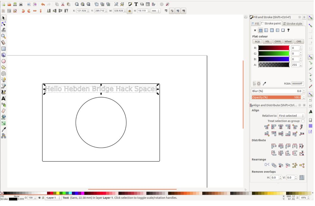
Text can also be added and aligned. We can also change the fill and stroke of text. When laser cutting text there should NEVER be a fill to it, only a stroke.
