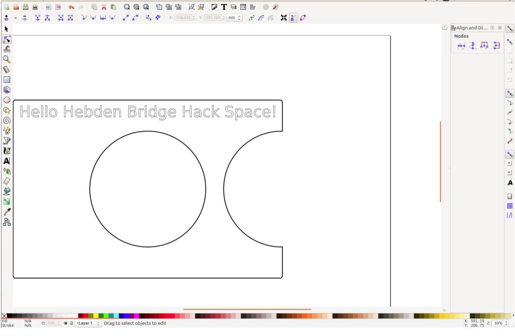
This is the difference of the original shapes. Select both using Shft+Ctrl+\*select  $1^{st}$  object\*+\*select  $2^{nd}$  object\* then Path > Difference
